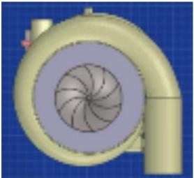
Centrifugal chillers are machines that use rotating impellers to compress the refrigerant vapor. Inlet vanes limit the flow of refrigerant to the rotor, which changes the amount of cooling that can be done. Most centrifugal chillers used today are powered by electric motors, but they can also be run by natural gas, diesel, or steam turbine engines.
