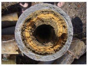
level of insoluble substances. As water leaves the system through evaporation and blow-down at the cooling tower, these solids become more concentrated in the condenser water system. When make-up water is used to replace the water lost through the tower, it brings in more solids.
