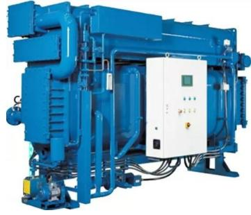
Absorption chillers are different from other types of chillers because they get their power from heat instead of from a motor. Absorption chillers can be either directly or indirectly lit. Direct-fired absorbers use natural gas or a similar fuel to make the heat that the unit needs to run. Indirectly fired absorbers get their energy from lowpressure steam, hot water,
