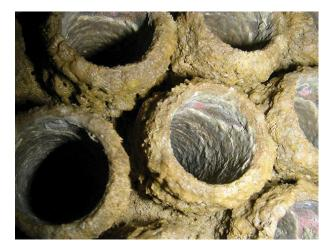
Solids that cause fouling can also come from the system itself. Metallic corrosion of pipes and erosion of surfaces let solids into the water system, where they stay in suspension until a chemical reaction makes them settle out, usually on surfaces that transfer heat.
