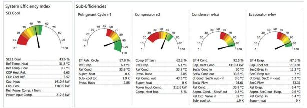
Data obtained by an advanced chiller monitoring system make manual logging obsolete and will flag performance drift and maintenance issues
