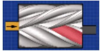
Screw Chillers are vapor compressor chillers that move the water through the system with the help of a screw compressor. Some of the most important benefits are small installation, quiet operation, lower costs for upkeep, and
