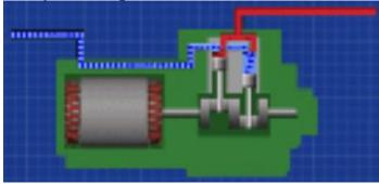
Reciprocating chillers are positive displacement blowers that use one or more pistons to squeeze a refrigerant gas. Almost all of them are powered by electric motors. In a system with more than one
