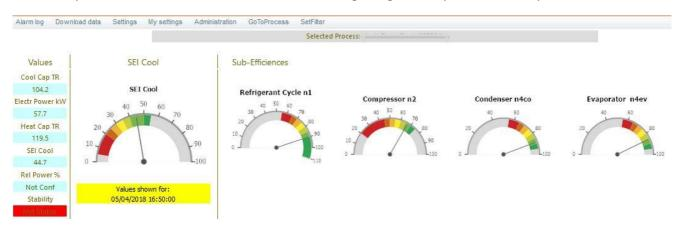
Performance at 50RT capacity is affected by poor part load performance of compressors. Part load results in poor compressor efficiency affecting total SEI that decrease from 45 to 30% representing a significant loss of efficiency as the chiller does not operate at high efficiency at the prevailing loads.
