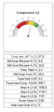
The compressors is operating with 58% isentropic compressor efficiency at stable operation were normal efficiency of these chillers are reaching around 70% at peak conditions and full load.
