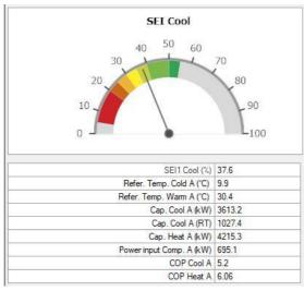
The total **System Efficiency Index** (SEI) is 38% which is lower than expected of high efficiency chillers at peak conditions full load.
