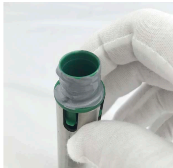
A cement ring forms around the holder.
