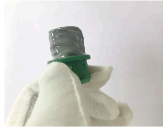
Socket with cement layer
