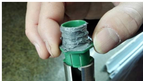
A cement ring forms around the holder.
