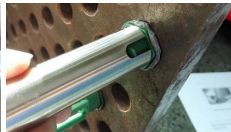
A cement ring forms around the holder.
