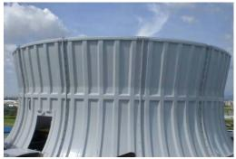
Fiber-reinforced plastic is the material of choice because of its light weight, durability and resistance to water. Design parameters conform to CTI standards. Available options include silencers, mesh guards and enhanced shapes to enable velocity recovery.
